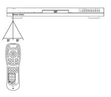
• The operating distance may vary according to the brightness and type of lighting in a room.
